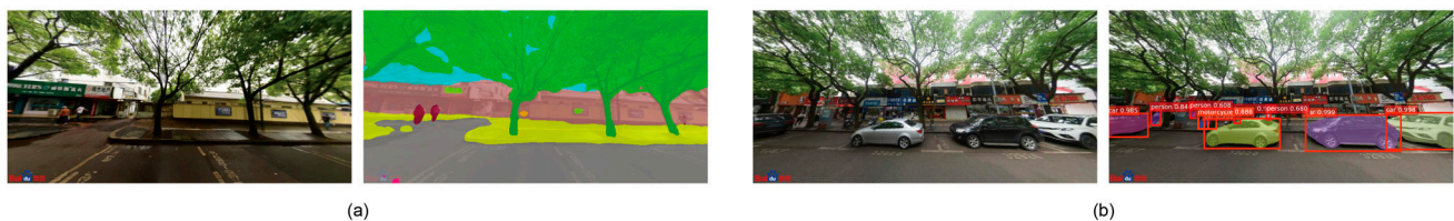
Figure 4. Examples of CV segmentation results. (a) DeeplabV3 semantic segmentation. (b) Mask R-CNN instance segmentation.
